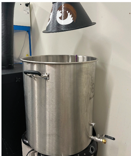
Figure 1.14 A kettle used for brewing beer is a great makeshift dye vat. These kettles have a spout and valve that can be attached to a hose in order to drain the spent bath.
